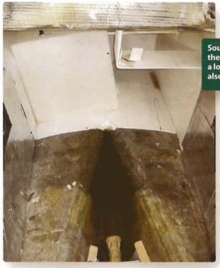
Sound and vibration insulation is particularly important on the propeller plane because drive components can generate a lot of noise. The fire retardancy of damping materials is also paramount in these areas.
