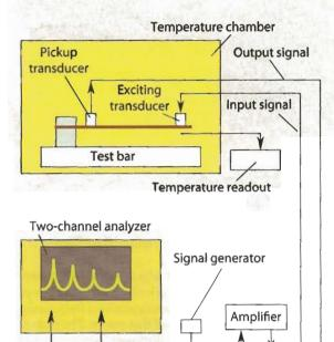
Within a temperature chamber, damping material is parasitically attached to a cantilevered steel bar to test damping response. A magnetic transducer excites the free end of a bar while a second transducer near the clamped end measures responses. A sound analyzer computes the transfer function and loss factor.
